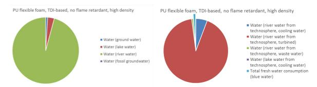
Figure 8: Total freshwater use (input), freshwater release (output) and freshwater consumption (TDI-based PU foam without FR, density 35 to 40 kg/m³)
