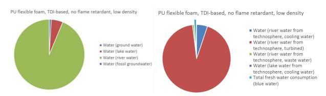
Figure 9: Total freshwater use (input), freshwater release (output) and freshwater consumption (TDI-based PU foam without FR, density 18 to 25 kg/m³)
