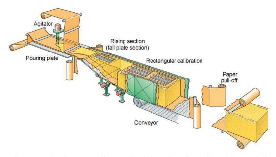
Figure 1: 3-D representation of a system – without metering device and cut-off saw – for continuous production of flexible rectangular foam blocks by means of the QFM process (source: Hennecke GmbH)
