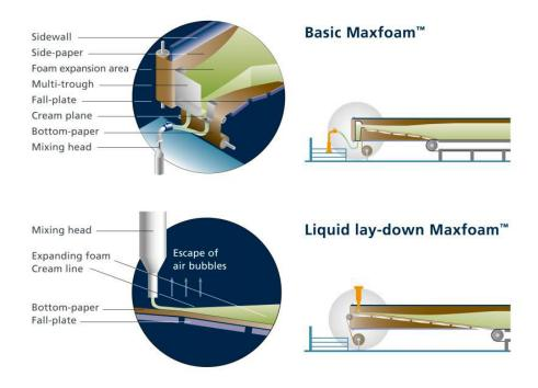
Figure 2: The Maxfoam production process (source: Laader Berg)
