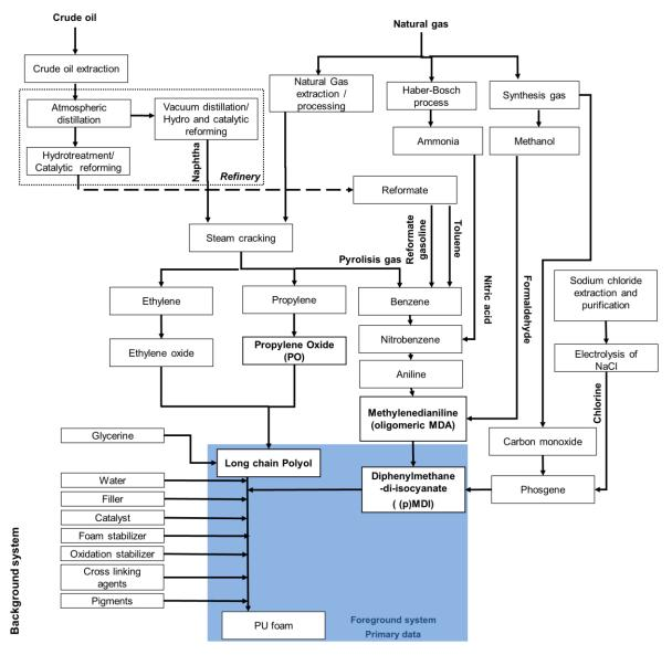
Figure 4: Cradle-to-gate system boundaries MDI based Flexible PU Foam
