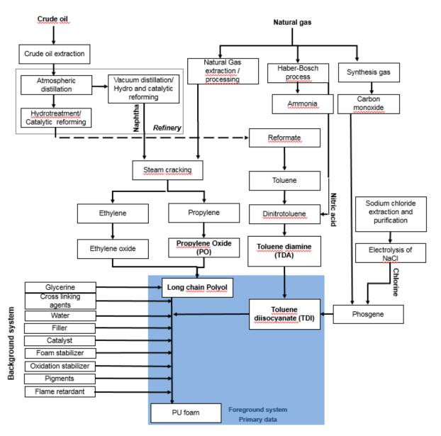
Figure 3: Cradle-to-gate system boundaries TDI based Flexible PU Foam
