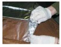
Roll the ends twice and press flat against the foam block
