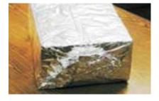
The finished foil wrapped sample should be tightly sealed on all sides.
