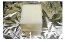
Place the foam sample in the center of the joined foil sheet lengthwise on top of the seam
