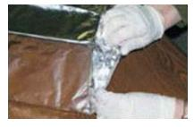
Roll the ends twice and press flat against the foam block
